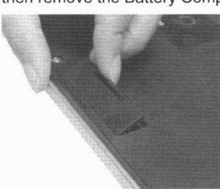
Install two AAA batteries into your keyboard following the battery orientation guide in the battery bay.
