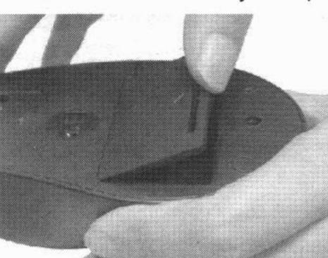
Install two AA batteries into your mouse following the battery orientation guide in the battery bay.
