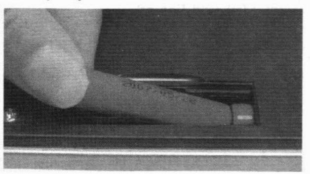
6. Replace the Battery Compartment Cover back onto your keyboard until it securely locks.
