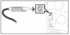
TIP: For most computers, the PS/2 Keyboard Port is located on the top of the back panel. If you are not able to find the PS/2 Keyboard Port on your computer, please refer to your motherboard's user's manual.
